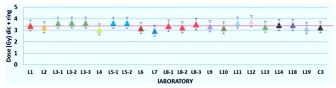
Figure 5. Doses estimated using the DCA-TC method (Dic + ring) from each of the partners compared to the physical dose of 3.27 Gy (red line). The error bars give the Poisson standard error on the estimated dose.
